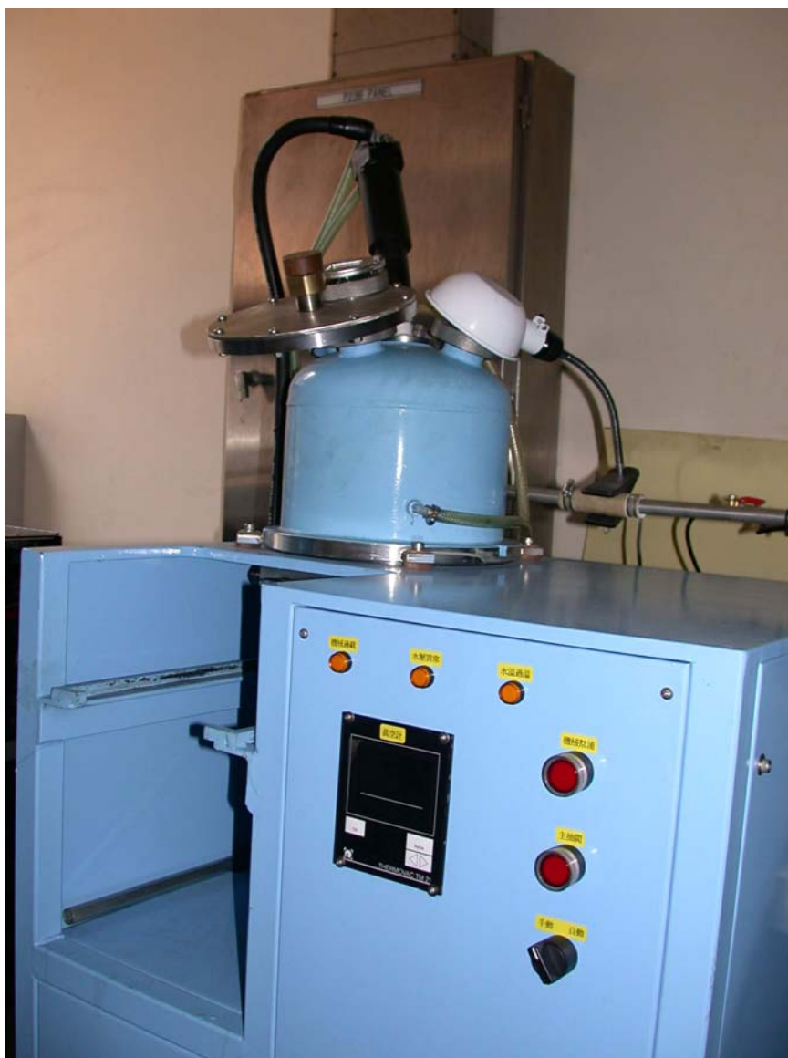
Figure 3.9 Photograph of the arc melting device.
